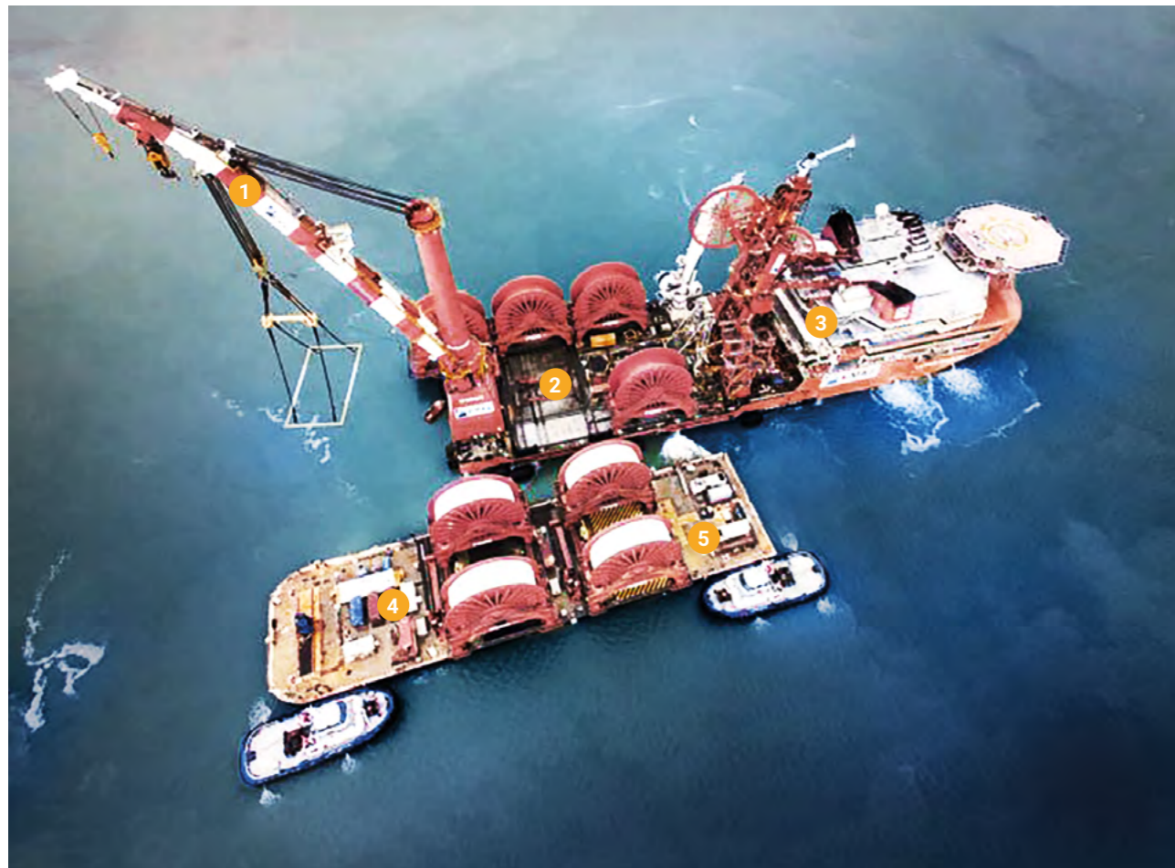
1 Controlling Load Moments 2 Combined Blower Heel Control and Roll Damping system 3 Loading Computer with Crane Operation Simulation 4 Heel Control system with Zero-Flow 5 Draft Measurement, Tank Content Measurement and Valve Remote Control system
