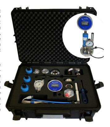
Nevertheless, at some point every component reaches the end of its lifecycle. This is the moment where HOSET 2.0 shows its advantages. Carrying up to three spare hydrostatic pressure sensors in a robust casing, HOSET 2.0 can be stored on board – always ready for sensor replacements.
